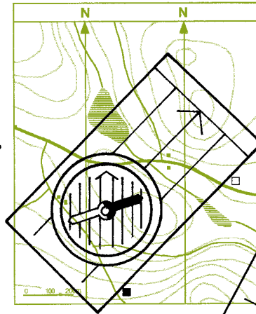
2. Turn the compass housing so it points North.
